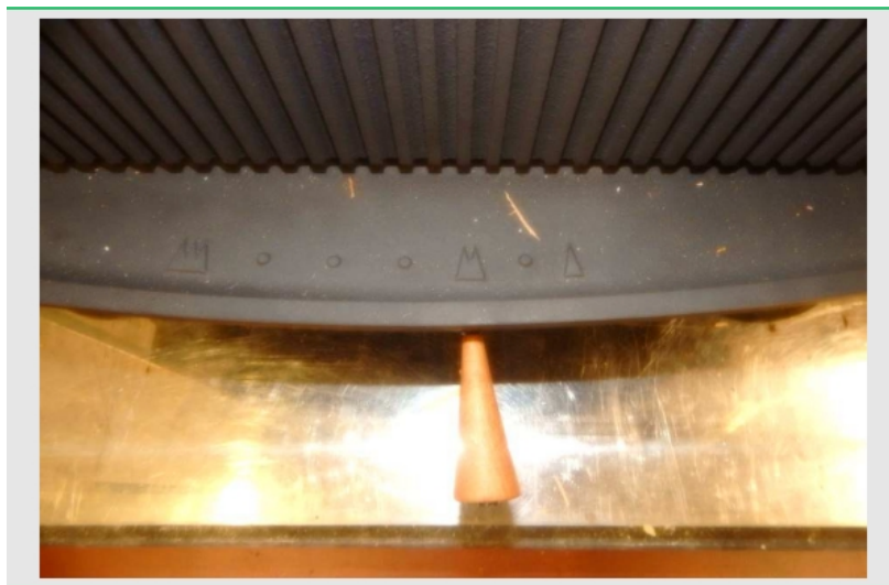
Setting of primary air control for performance tests at nominal heat output
