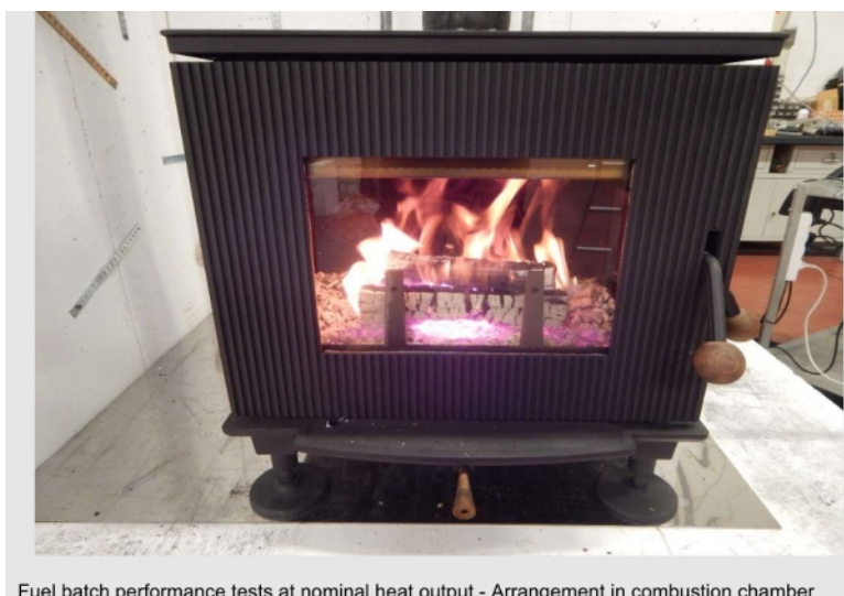
Fuel batch performance tests at nominal heat output - Arrangement in combustion chamber
