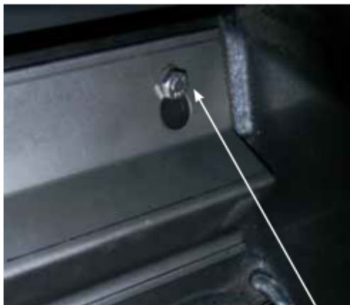
Ensure deflector is seated so bolts are situated at the top of the keyhole before tightening. Hand tighten bolts only.
